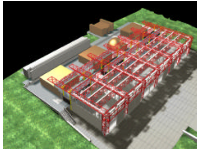
Figure 4. Isometric of proposed facility showing structural elements
